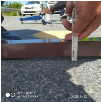
Figure 2. "Lath" with measurements taken 75m from the intersection
