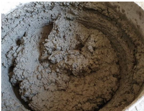
Figure 4. Rubberized concrete that is ready to be cast
