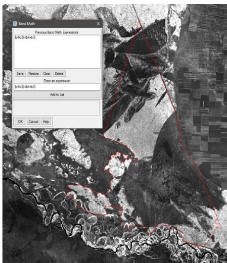
Figure 5. The process of the NDVI calculation The scale of the vegetation density map in the Zhanasemey branch of the GLPR Semyey Ormany is 1:200 000.
