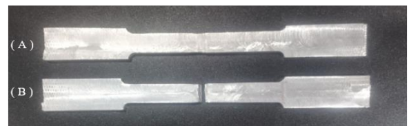
Figure 1. The specimen used in the tensile test; (A) before and (B) after the test
