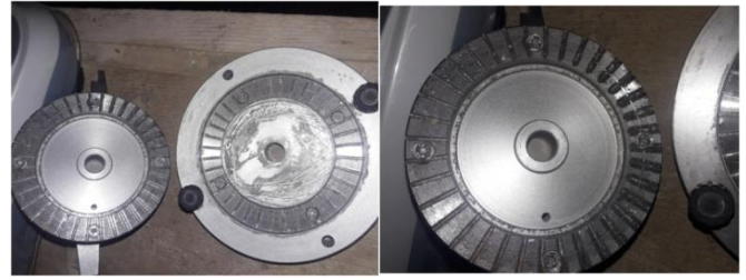
Figure 3. Top and bottom steel discs to simulate the steel silo wall
