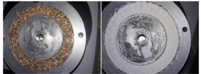
Figure 4. Wheat and Wheat flour in the ring shear box
