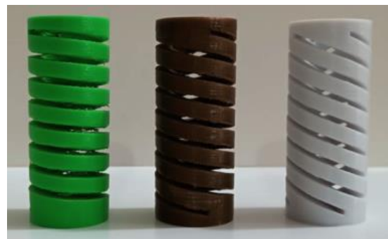
Figure 4. Spring with one, two, and four coils (octet infill pattern and 100% infill percentage)
