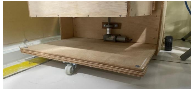
Figure 17. Testing DC motor with lead screw
