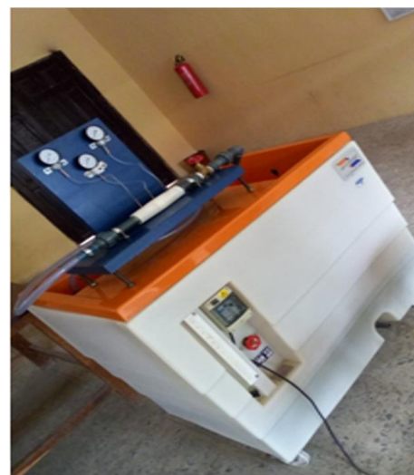
Appendix 2. Bernoulli's apparatus on hydraulic bench
