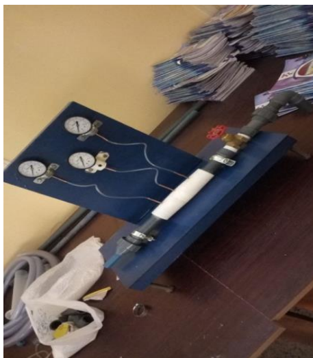
Appendix 1. Bernoulli's apparatus assembly
