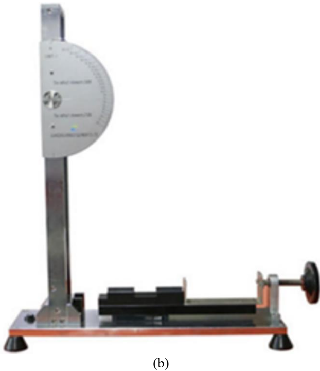
Figure 2. (a). Schematic diagram for spring hammer calibration device using pendulum in accordance with IEC6006-2-75, (b). Photo for the spring hammer calibration device describing positioning of the spring hammer [7]
