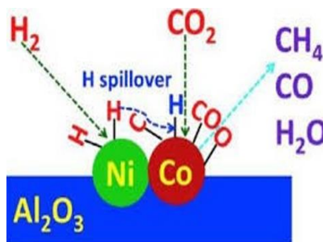
Figure 2. Hydrogenation of CO 2 coproduced with biomethane
