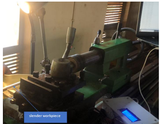
Figure 10. The setup and the process of the cutting test on the slender workpiece
