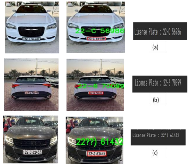
Figure 13. The ambiguous recognition of characters (a) recognizing (0 as 6) (b) recognizing (G as 6) (c) recognizing (J as)
