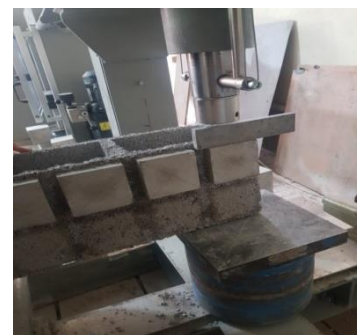
Figure 3. Lap-shear adherence test of mortars
