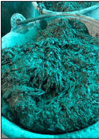
Figure 6. New complex synthesis of concrete with WP fibers [92]
