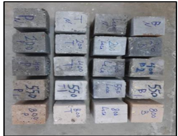
Figure 10. The color change in four types of lightweight Geo-Polymer concrete after exposed to (35, 200, 400, 550, 800°C) (Own source)
