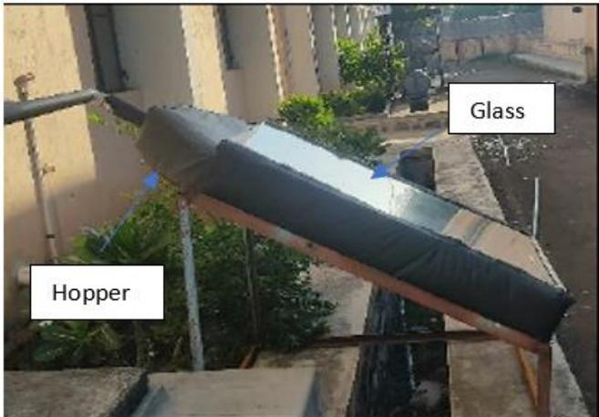
Figure 4. Solar flat plate collector at site
