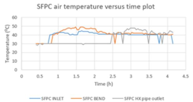
Figure 6. Time vs temperature of SFPC piping
