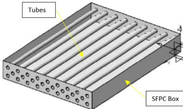
Figure 5. Tube arrangements in SFPC
