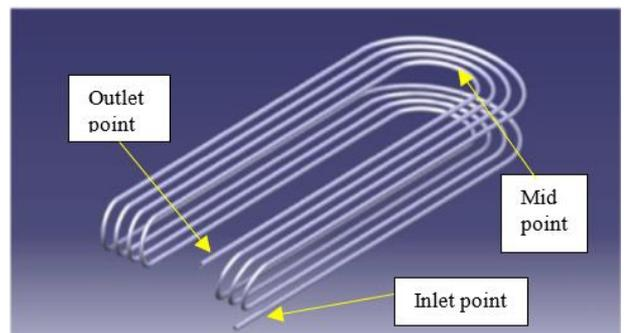
**Figure 3.** Temperature measuring locations on HX tubing for TES
