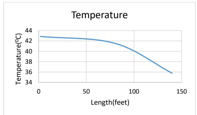
Figure 7. Temperature profile in the TES
