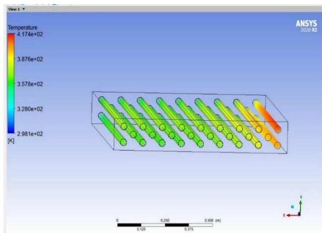
**Figure 8.** CFD simulation of flow through SFPC
