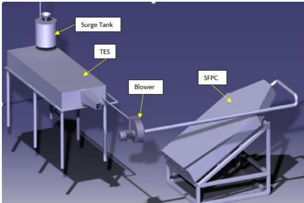
**Figure 1.** Experimental set up of SFPC-TES
