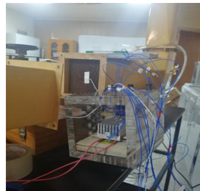
Figure 3. Heat sink inside the test section of the wind tunnel
