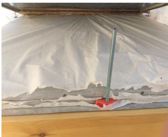
Figure 4. Wick in loose contact with galvanized steel plate
