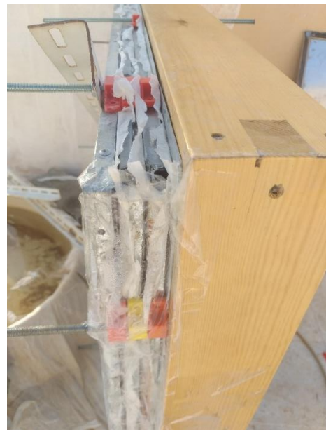
Figure 5. Side view of distillation unit with 3 effects. A duct tape was used to reduce vapor leakage and heat loss
