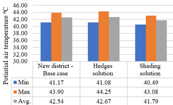
(a) Max, min and average potential air temperatures for the base case and the solutions
