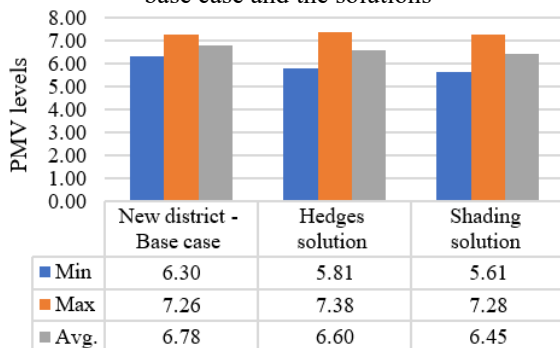
(b) Max, min and average PMV levels for the base case and the solutions
