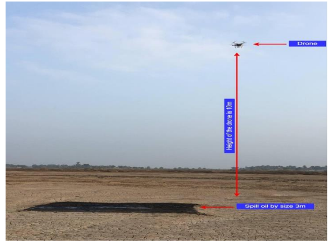
Figure 8. Drone taking images of the oil leakage
