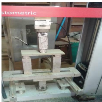
Figure 4. Flexural strength test set up for the composite tiles
