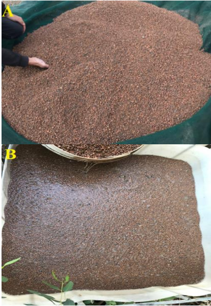
Figure 1. (A) LECA was drained in the laboratory air; (B) LECA was soaked in water
