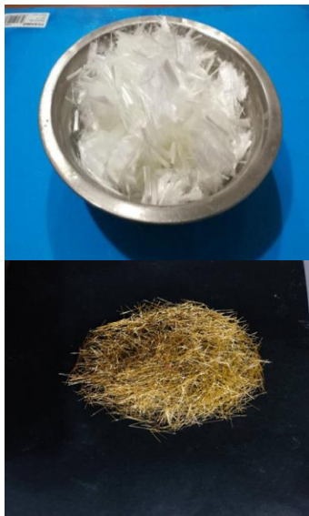
Figure 2. Micro steel and polypropylene fibers used in this study
