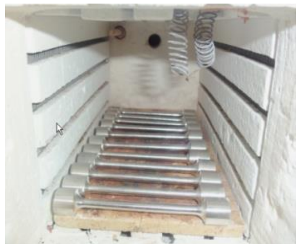
Figure 2. Arrangement of test specimens inside the oven
