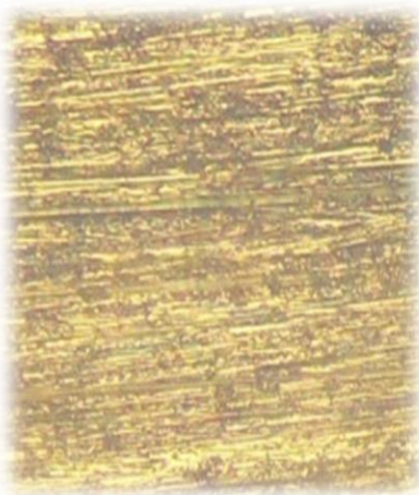
Figure 18. Annealed specimen deformed at 33% (periphery zooms X40)
