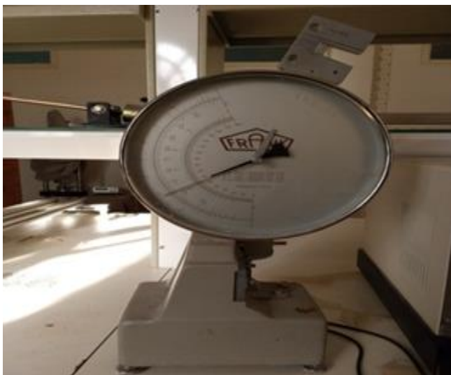
Figure 6. Pendulum impact tester-for 4J
