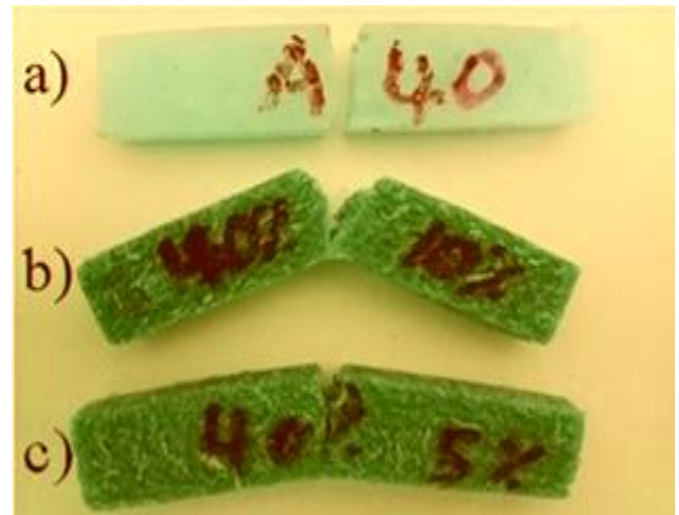
Figure 9. Appearance of the overall shape of the effect samples 40% glycerol earlier than and after reinforcement (a. MC40 bioplastic; b. MC40/OP5 bio composite; c. MC40/OP10 bio composite)
