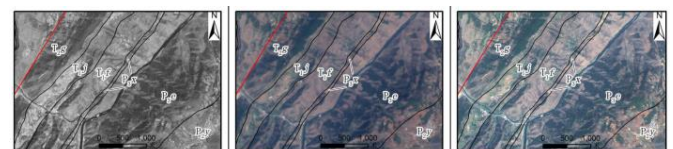
Figure 10. Comparative visualization of the 1:50000 mapping effect for remote sensing geological element identification - Panchromatic image (left), Multi-spectral image (middle), Fused data image (right)
