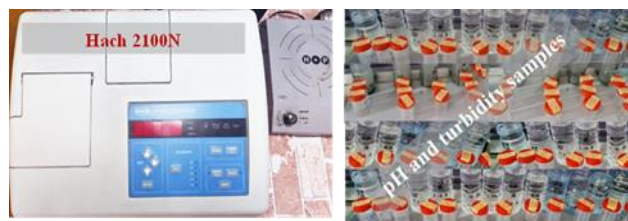
Figure 12. Turbidimeter instrument and samples
