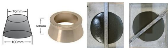
Figure 3. Filling ability of NDRPC
