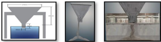
Figure 2. Flowability test of NDRPC
