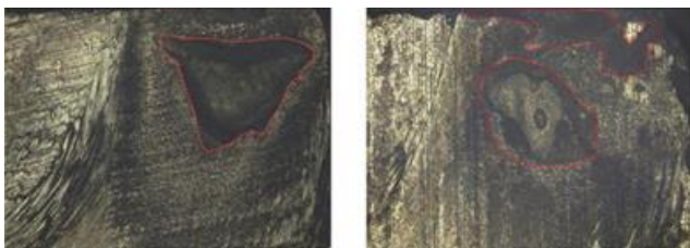
Figure 6. Bond breakage morphology on tool-chip interface
