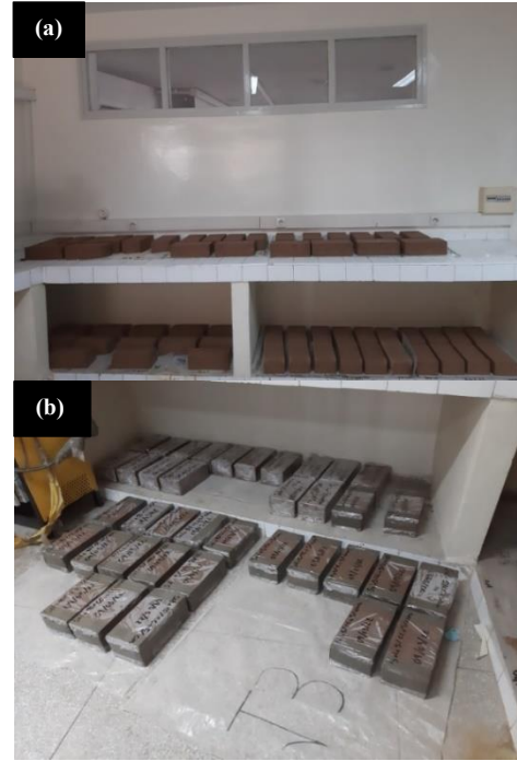
Figure 12. Storage and curing of (a) non-stabilized blocks, (b) cement stabilized blocks
