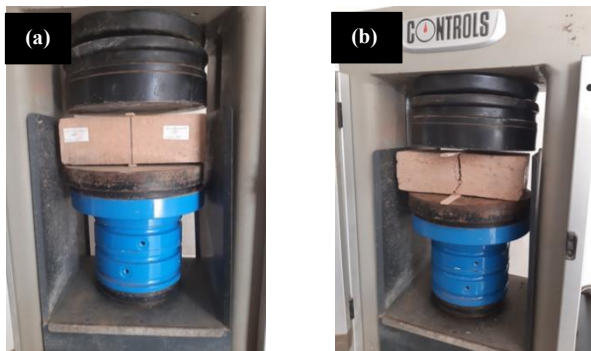
Figure 15. Splitting tensile strength test
