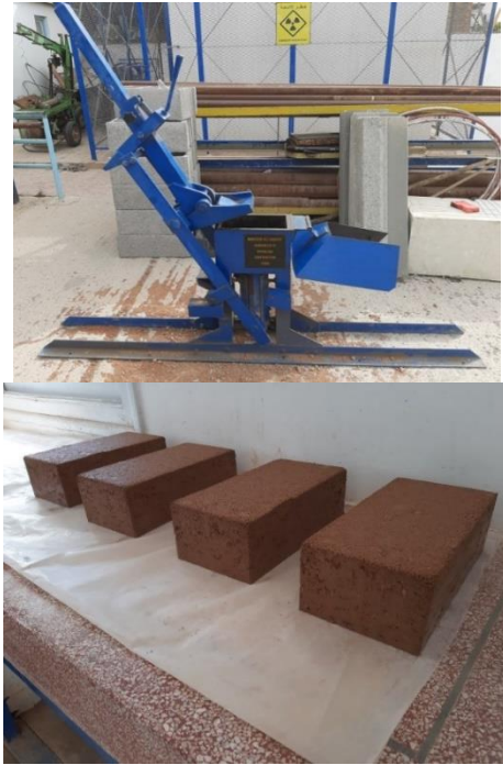
Figure 10. Compressed earth blocks manufacturing
