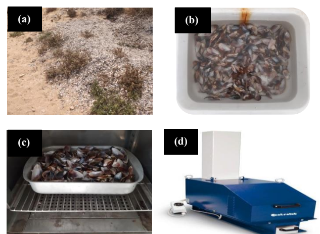
Figure 6. Preparation of mussel shell aggregates (a) Cap Ghire site, (b) mussel shell washing, (c) mussel shell drying, (d) jaw crusher
