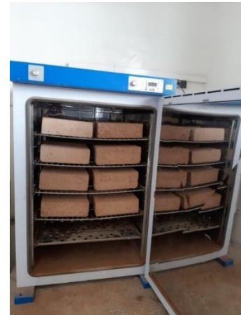
Figure 13. Drying of manufactured blocks
