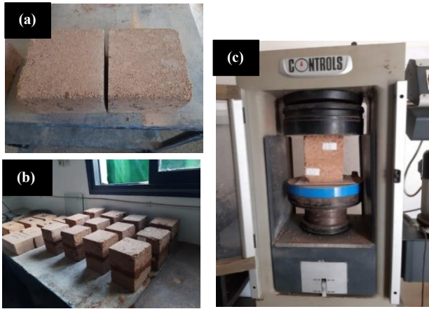
Figure 14. Dry compressive strength test; (a) cutting the block into two half-blocks, (b) superposition of the two half-blocks, (c) set up used for dry compressive strength
