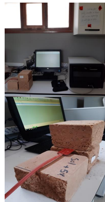
Figure 17. Thermal conductivity measurement of CEB using the Hot Disk Thermal Constants analyzer
