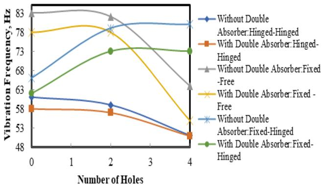
**Figure 10.** Effect of the double absorber, number of holes, and end conditions on the vibration frequency
