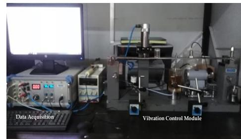
**Figure 2.** Vibration fundamental trainer
