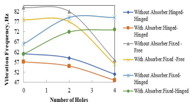
**Figure 9.** Effect of single absorber, number of holes, and end conditions on the vibration frequency
