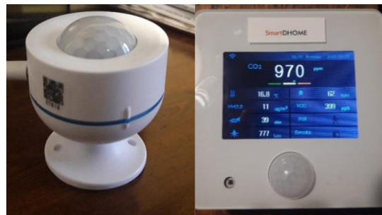
Figure 3. Smart monitoring sensors used for measurements
