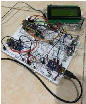
Figure 4. Integrated wiring of client and server systems
