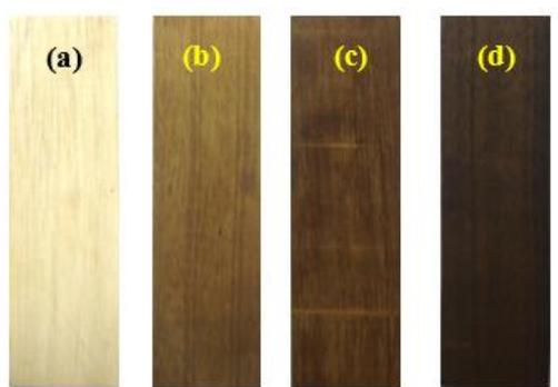
**Figure 2.** The look of jabon wood after being subjected to oil heat treatment at varying temperatures: (a) untreated sample, and heat-treated samples at (b) 170°C, (c) 190°C, and (d) 210°C
