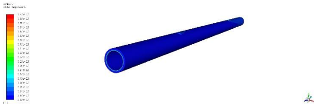
Figure 17. Static temperature contours for Re (24000), smooth tube with baffle, d=20 mm
