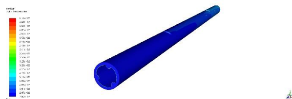
Figure 14. Static temperature contours for Re (24000) with rod baffle, G.T(3-star)
