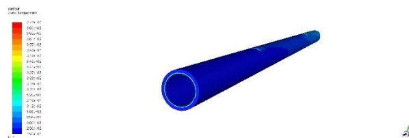
Figure 16. Static temperature contours for Re (4000), smooth tube with baffle, d=20 mm
