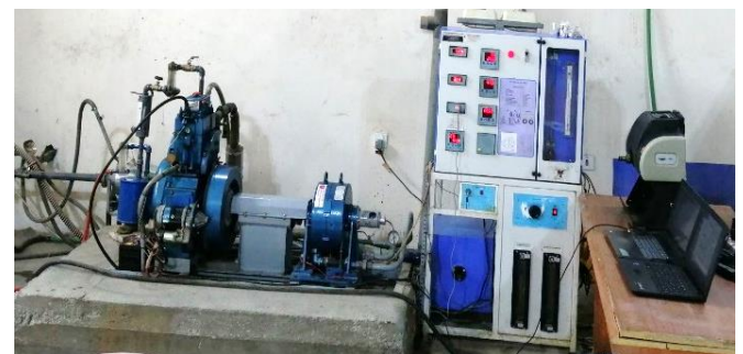
Figure 3. The layout of the diesel engine experimental setup
