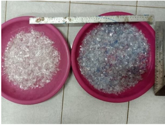
Figure 4. PET and PP plastic waste sample using in the research before grinding process
