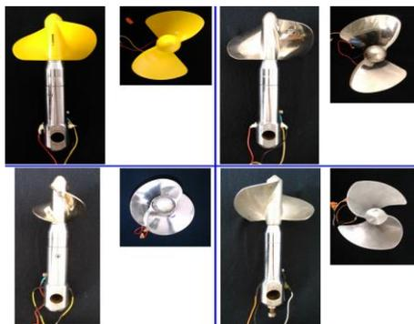
Figure 1. Typical current meters (propellers are manufactured by Ott and GMP) used by IMP PAN
