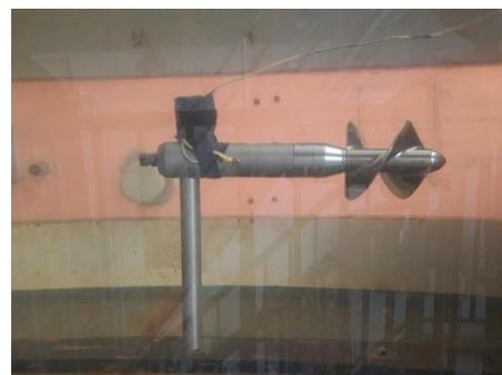
Figure 4. The 80mm diameter current meter in the measuring chamber: reverse setting
