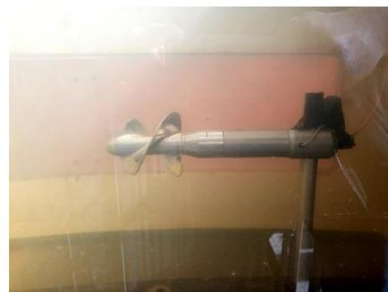
Figure 3. The 80mm diameter current meter in the measuring chamber: standard setting
