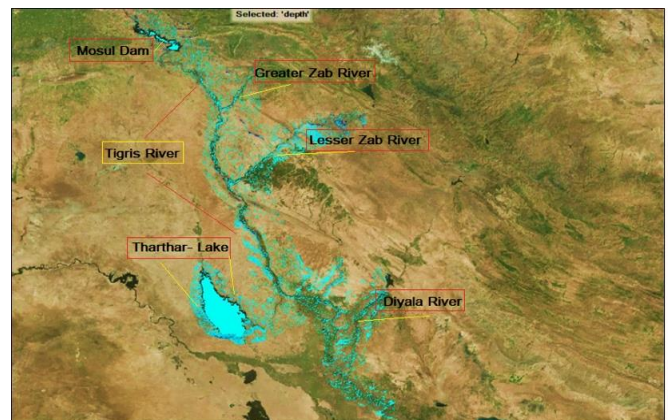
Figure 10. Expected Runoff-Depth for 100 years return period simulated by HEC-RAS model in Tigris River basin
