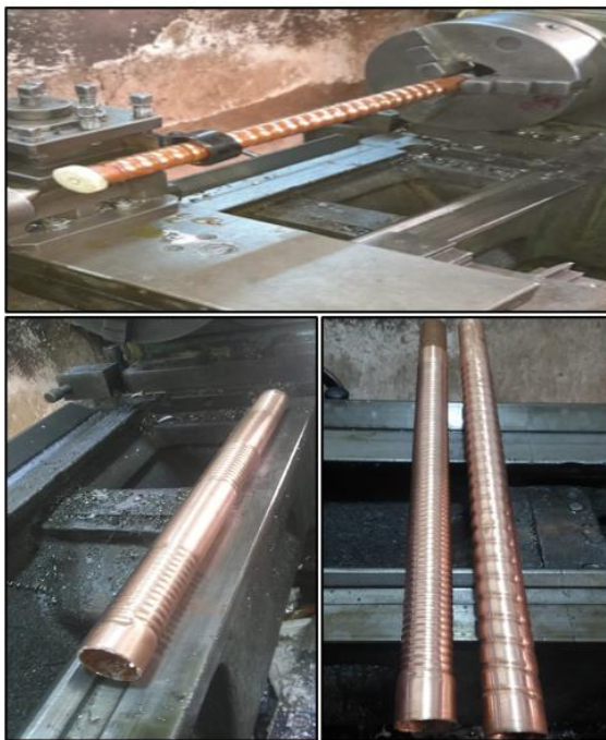
Figure 4. Manufacturing of corrugated tubes models
