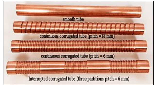
Figure 5. Tested copper tubes
