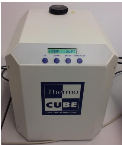
Figure 3. Recirculating chiller system
