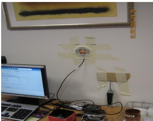
Figure 1. Internal measurement equipment for heat flow rate, surface temperature, and air temperature (Francesco Passerini, 2016, picture taken by an author of this paper in the context of the here presented research)
