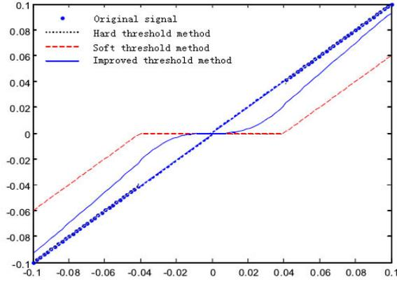
**Figure 2.** Illustration of the three threshold functions
