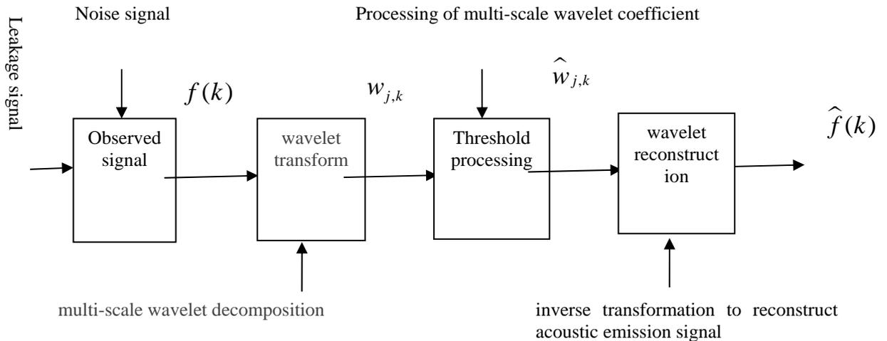
Figure 1. Scheme of realizing the improved threshold denoising method
