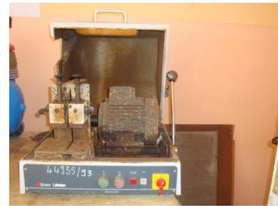
**Figure 1.** Chainsaw for cutting (struers labotom)
