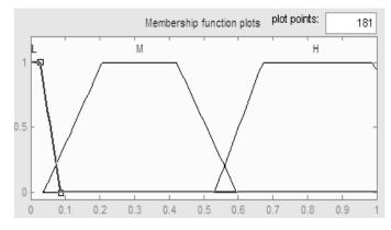
Fig.3. Membership functions of input variable
