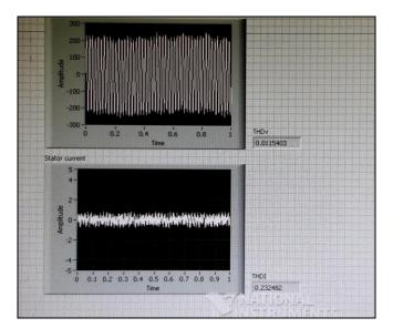
Fig.6. Stator Voltage and Current Waveform in LabVIEW
