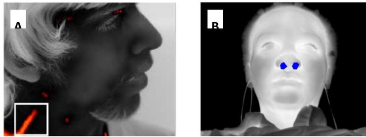
**Figure 3.** Temperature fluctuations of (A) carotid and (B) nostrils are continuously monitored to respectively measure pulse rate and breathing rate in thermal images. Modified from [10]
