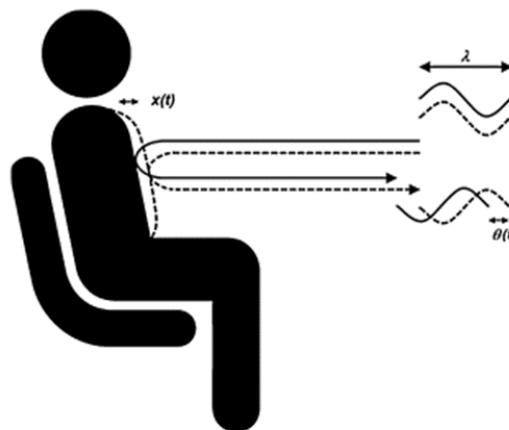
**Figure 2.** Pulse rate and breathing rate engender unintentional movements of the chest. These displacements can be sensed by the Doppler effect. The frequency and the phase of the reflected signal are slightly different from those of the source signal. From [3]
