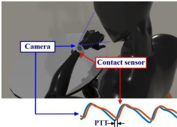
**Figure 6.** Pulse Transit Time (PTT) corresponds to the time the pulse wave takes to travel from one point of the arterial tree to another. In this example, PTT is computed using PPG waveform analysis of face and wrist. The physiological signals are recorded with a contact sensor (for measuring wrist signal) and a camera (for measuring face signal), both sensors being embedded in a smartwatch. From [39]
