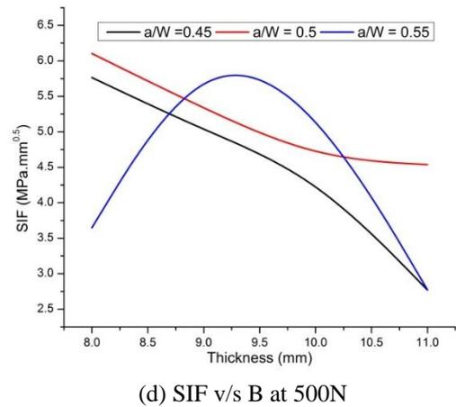
**Figure 4.** Variation of SIF with thickness for different crack lengths
