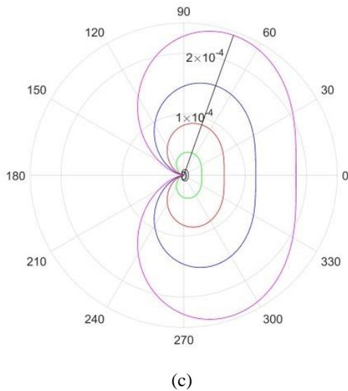
**Figure 7.** Shape of plastic zone for different crack length and 100N load
