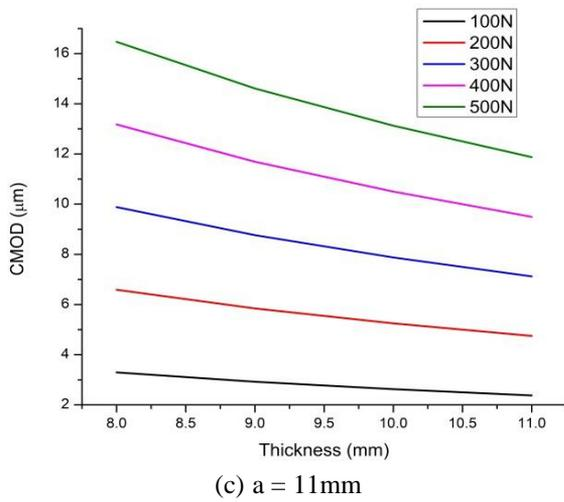
**Figure 3.** Variation of CMOD with thickness
