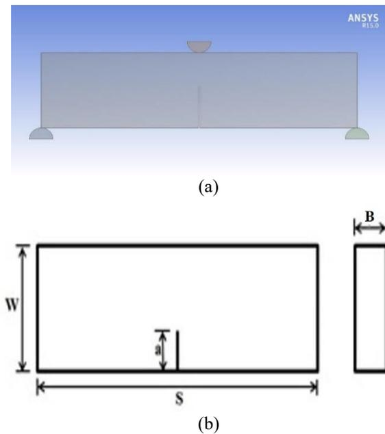
Figure 1. Geometry of the specimen
