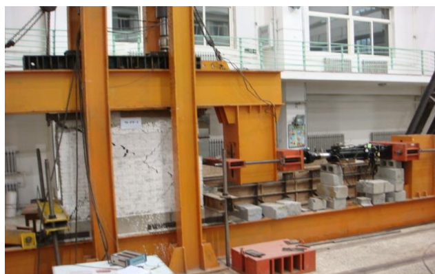
Fig.1. Picture of Loading Devices of The Test
