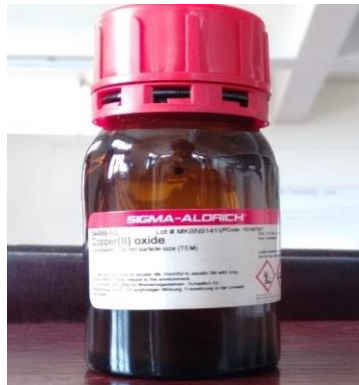
Copper oxide nanoparticles of size <50nm
