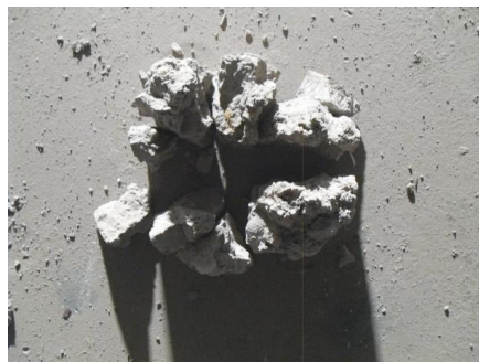
Fig. 10. Radial fracture of experiment 3.
