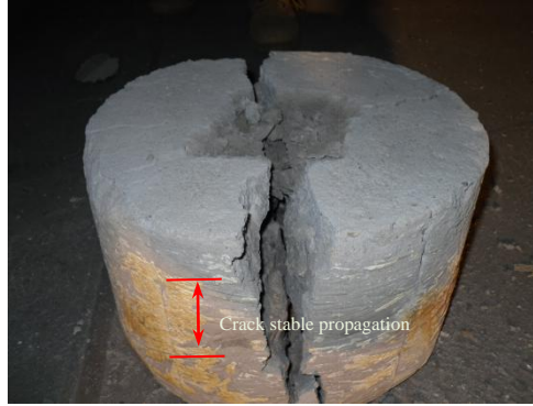
Fig. 13. Splitting crack propagation of experiment
