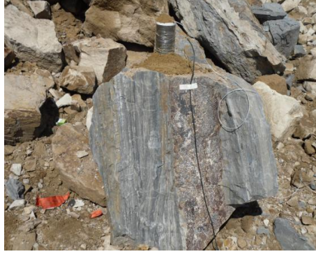
Fig. 15. Placement of the linear shaped charge structure.
