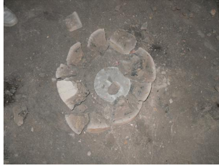
Fig. 11. Radial fracture of experiment 4.
