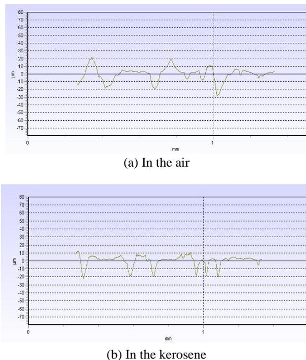
**Figure 9.** Roughness curve of ceramic discharge pits
