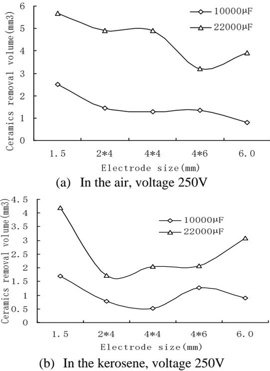
**Figure 6.** Effect of electrode size to ceramics removal volume based on capacitance
