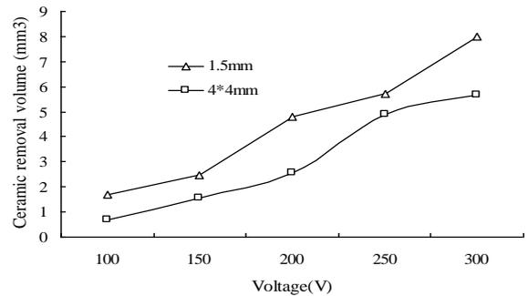
(a) In the air, capacitance 22000 $\mu\text{F}$
