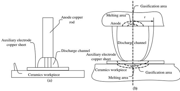
**Figure 1.** Schematic diagram of impulse discharge on capacitor
