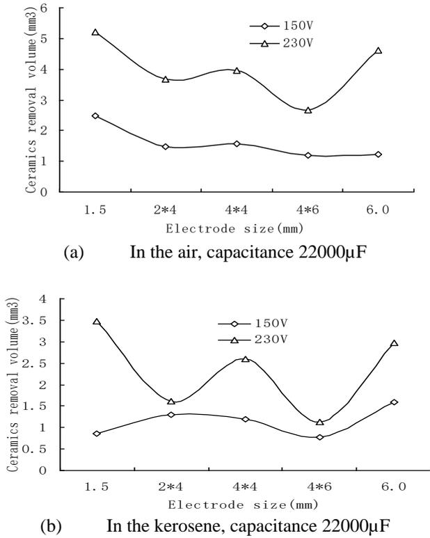
**Figure 5.** Effect of electrode size to ceramics removal volume based on voltage
