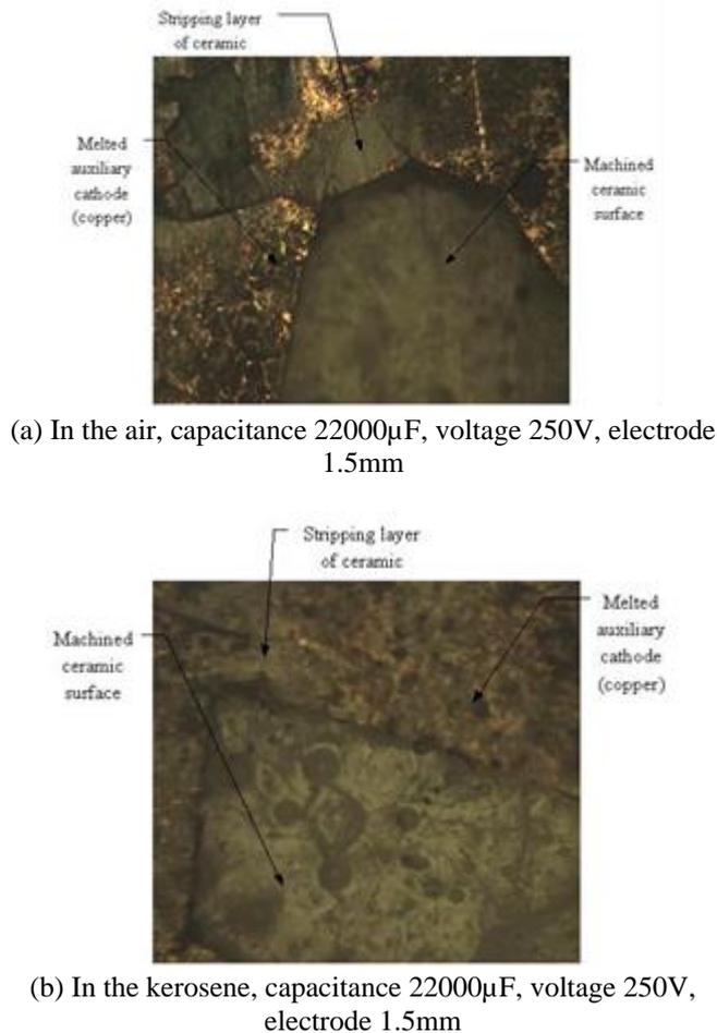
**Figure 8.** Micrograph of EDM ceramics surface by X 200 Metallography
