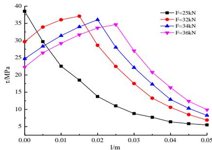
**Figure 6.** Shear stress distributions of the bolts at different loads
