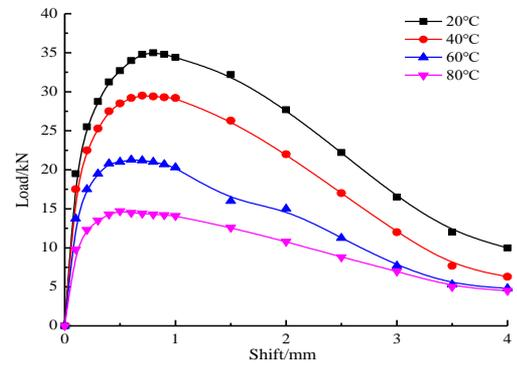
**Figure 4.** Load-displacement curves at different temperatures
