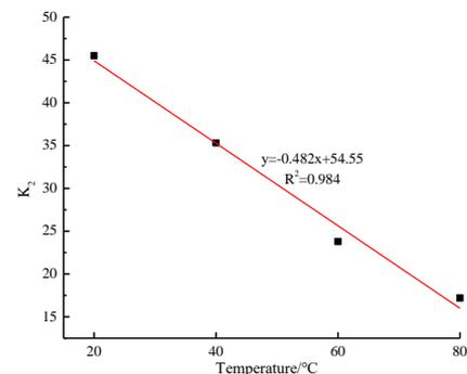
**Figure 5.** Relationship between tensile shear stiffness and temperature
