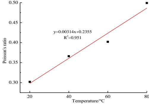
(b) Poisson's ratio and temperature
