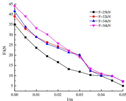
**Figure 7.** Axial force distributions of the bolts at different loads
