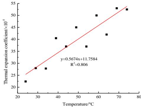
**Figure 3.** Thermal expansion coefficients of the bolting system at different temperatures
