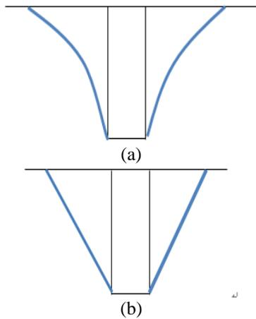
**Figure 1.** The shape of the failure surface of the shearing cone
